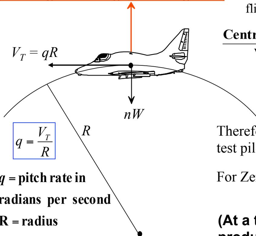
$$\frac{\text{Centrifugal Force}}{\text{Weight}} = n_a = \frac{WV_T q}{Wg} = \frac{V_T q}{g} = n - 1$$
